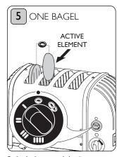
2 & 4 slot models: Rotate the 'selector switch' anticlockwise to the one bagel symbol. Only the second element from the left will heat up.
